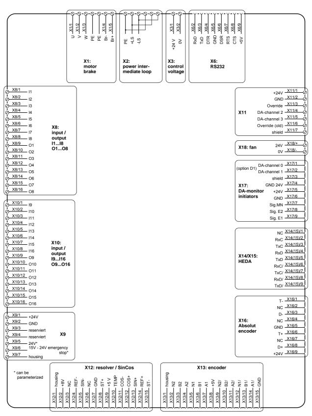
The assignment of X12 does not apply for the S3 option.
